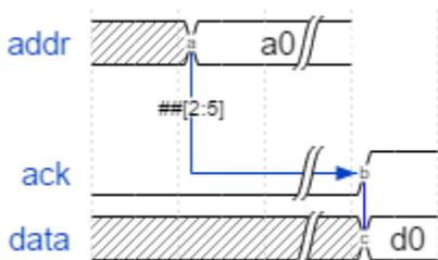
The dot character (‘.’) in Wavejson means repetition of the value of the previous cycle, which naturally maps to the SystemVerilog \$stable construct.
