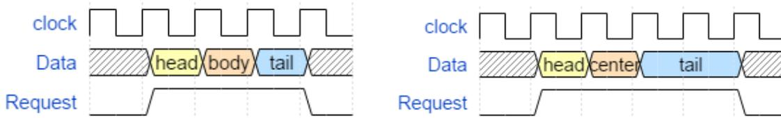
Similarly, when a simulation or logic analyzer dumps a large amount of trace data as text, it is difficult to understand the diff in context. As long as the trace dump is in WaveDrom format, or can be easily converted to WaveDrom format by a script, then rendering the waveform as an image and looking at the point of the difference makes it much easier to understand.
